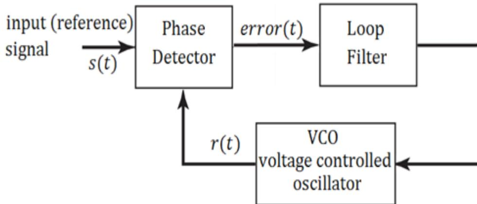
**Fig.1. Block diagram of the PLL**
