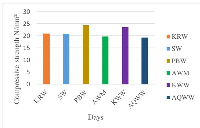
**Compressive Strength Analysis for Concrete Samples Produced and Cured for 28 Days:**
