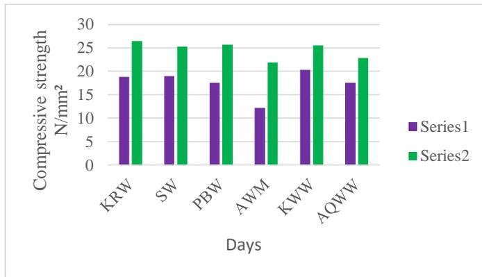
The difference in ACS between the earliest strength and the latest strength development is presented in Figure 6. The Amissano well water recorded the highest strength difference (9.700N/mm<sup>2</sup>) and was followed by the pipe borne water (8.127N/mm<sup>2</sup>) and the Kakum river water (7.593N/mm<sup>2</sup>). The least was recorded by the Kakumdo well water.
