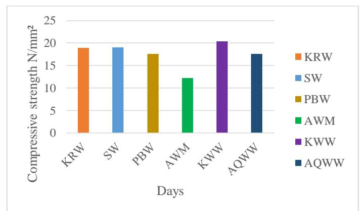
**Compressive Strength Analysis for Concrete Samples Produced and Cured for 14 Days:**
